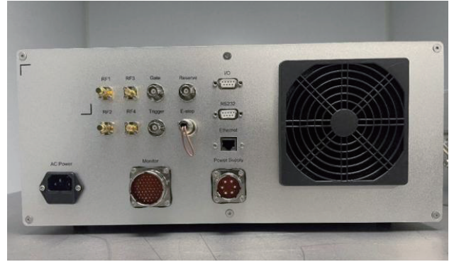
* Rear panel interfaces of the electric control cabinet
