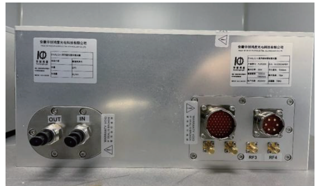
* Rear Panel Interfaces of Laser Head
